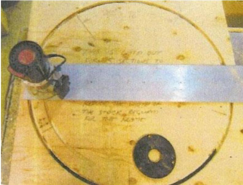
**2:** With a straight bit mounted to the router, cut the pattern ring out of Masonite, MDO or MDF board. You will not need to have a plunge router, an ordinary one will do. Just go slowly and increase the depth of cut until breakthrough. Cut the outside of the ring first and then the inner.
