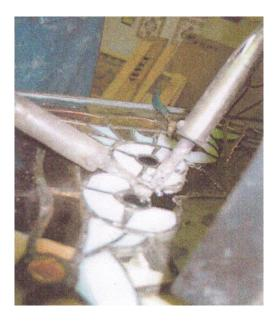
Step 1. Support the panel on blocks to allow solder to melt away. Use two soldering irons to provide plenty of heat over a long stretch of solder seam.
