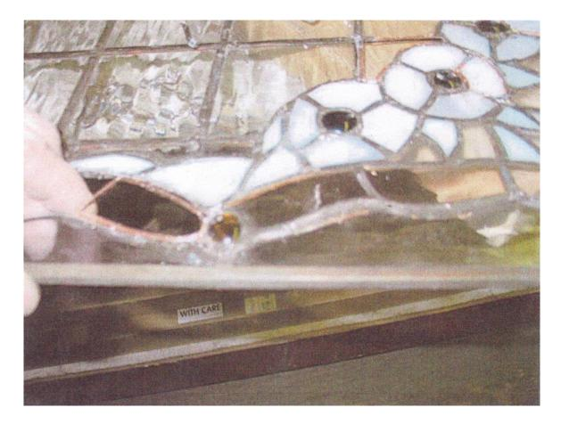
Step 3. Grind the new piece to a close fit, and after wrapping it with copper foil, solder it in place. Finish the top side first; the bottom will be a rougher-looking job when you first turn it over, but easier to solder if you've completed the top side first.
